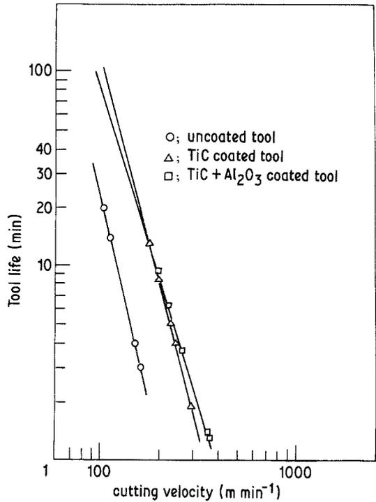
Figure 4  $T-V$  relationships for uncoated, TiC coated, and TiC + Al<sub>2</sub>O<sub>3</sub> coated tools using Taylor's method.
